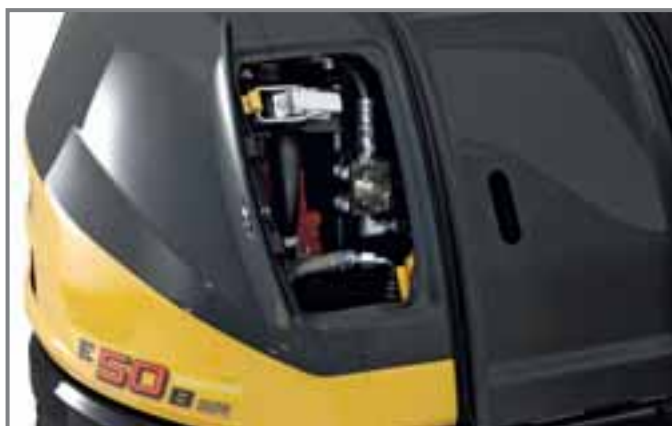
Easy and quick access to the selector of auxiliary circuit: mono- or bi-directional.
