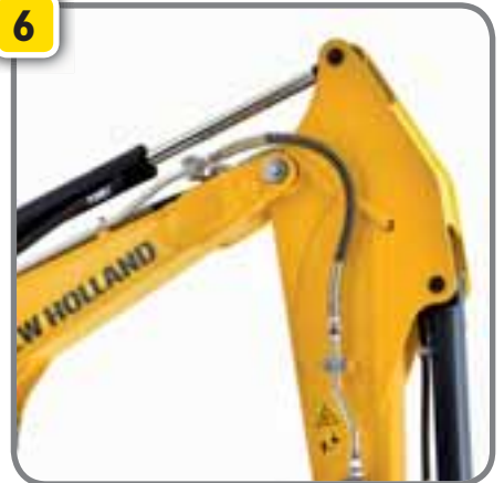
Reinforced boom/arm connection
