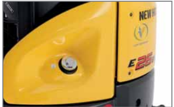
Fuel tank can be easily filled from the ground.
